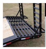
The 14DF is equipped with a 36" cleated dovetail for maximum traction and less slippage when loading and unloading equipment.
