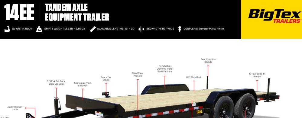
2-5/16" Demco BigTex EZ Latch Adiustable Coupler ST235/80R16 , Radial Tires 7K Axles Treated with Forward Pine Deck Self-Adjusting Brakes 6" Channel Wrap Also Tongue Avalaible with 4' Stand-Up
